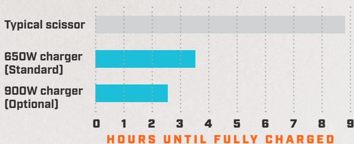
**Quick charge:** 5 min. of charge provides 100-ft of driving and enough torque for loading.
